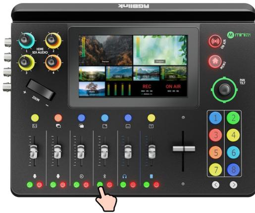
The left one is for simultaneous audio management of four HDMI / SDI signals on Program output port and Preview output port.
