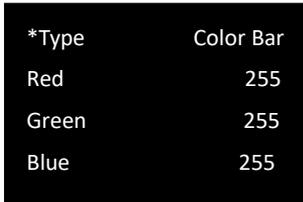
**Type:** Users can choose OFF to disable test Pattern, or choose any one from the following test patterns: Pure Color, Color Bar, V Color Bar, Ramp, Red/Blue, Checker, Window, Crosshatch, Slide Bar, Frame, T 32 Dots, T 64 Dots 5, T64 Dots 3, H Stripe, V Stripe
