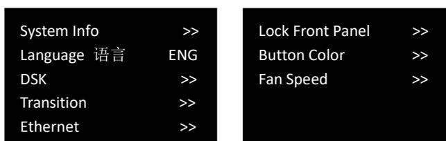
1) **System Info:** Show MCU version, Serial Number, and IP address of the device.
