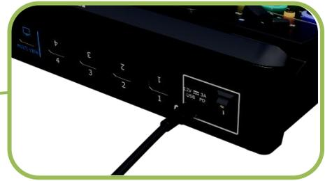
Connect mini-edge to power plug by the link cable
