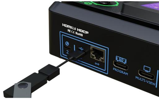
Insert a U disk to USB port labeled number 1. Before recording, format the U-disk first.
