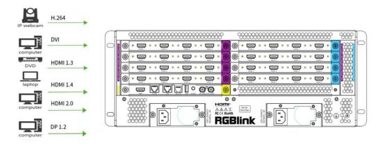
Q16pro series supports HDMI, DVI, SDI, DP1.2, HDBaseT and other optional input modules. Connect Q16pro with IP Camera, PC, DVD, laptop and other device as shown in the figure above.
