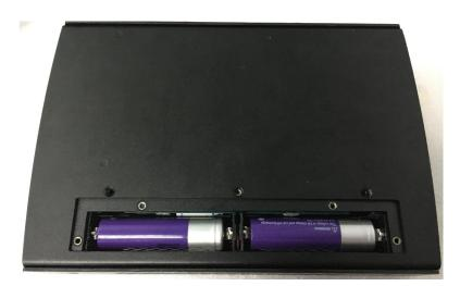
4. Install the holder, and lock the 7 screws, installing batteries is finished. As shown in the figure below:
