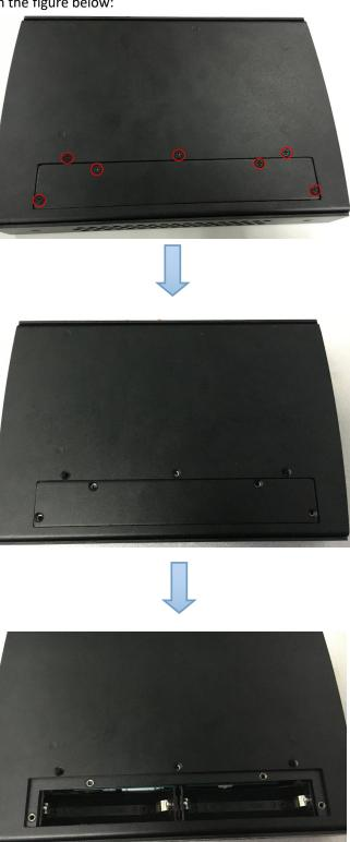
2. Prepare 2 lithium ion batteries. Pay attention to the positive and negative terminals of the batteries, this is the main points in installing the batteries. As shown in the figure below:
