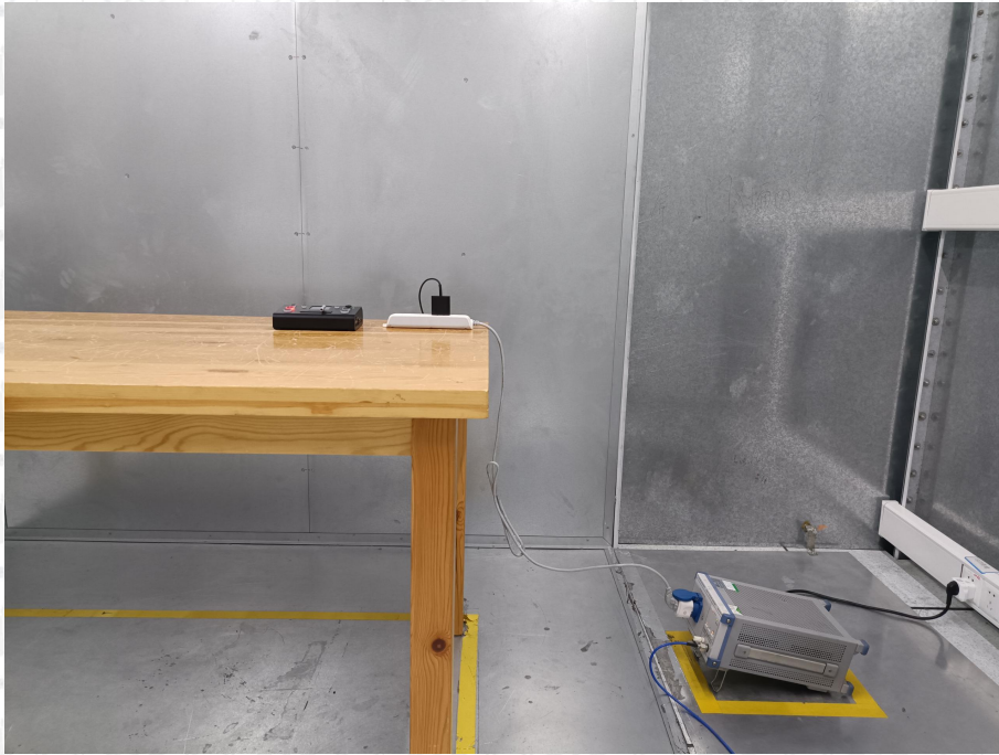
Figure 3: Conducted Emission Test Setup
