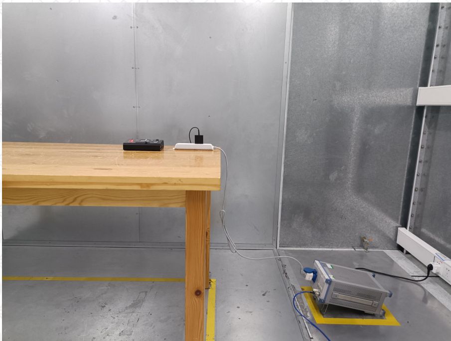
Figure 2: Conducted Emission Test Setup
