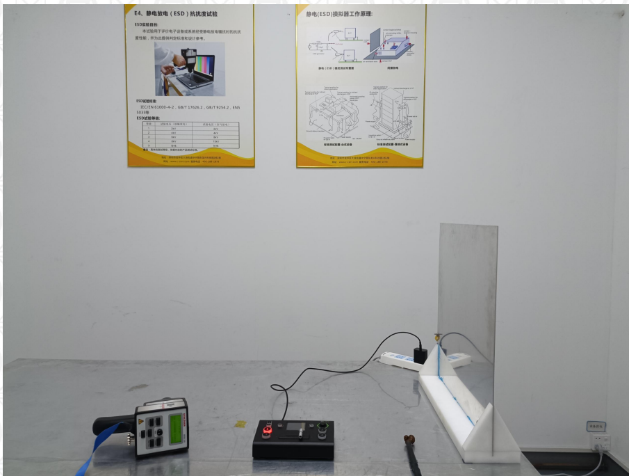
Figure 4: Electrostatic Discharge Test Setup
