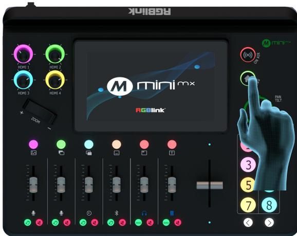
Push the MENU button and the 5.5-inch LCD screen will quickly enter the main menu interface. The right part of the screen displays the main menu interface, as shown in the right figure.
