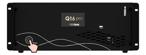
After connection, slightly press the power button in the front panel to turn on Q16pro.
