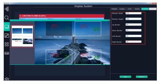
Parameter of Monitor Width, Height, Up Down Left Right Border are to set the overall monitor Display Area, not not single monitor, but the bar under is for single monitor.
