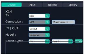
2.1. After X14 is dragged into the topology diagram interface, users can find how many X14 devices currently linked in the same network from the drop-down arrow after SN.
