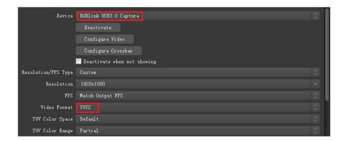
If there is no video format YUY 2 after setting above, check the USB 3.0 port connection. Make sure it is linked to USB 3.0 port on PC by USB 3.0 cable. (USB 3.0 cable or port is standard in blue while USB 2.0 is in black
