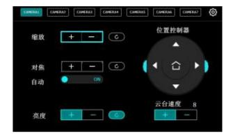
Zoom: Click [+] on the touch panel to zoom in the partial picture of the camera, and click [-] to zoom out Focus: The system defaults to auto focus. If manual focus is needed, the auto focus function can be turned off Brightness: Adjust the brightness of the camera
