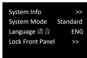
1. **System Info:** show MCU version,Serial Number, and IP address of the device.
