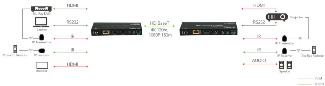
MSP 415 System Connection Diagram
