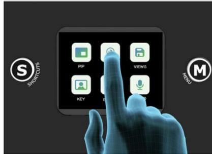
When you want to control PTZ camera, the IP address of mini-pro and camera should be in the same network segment. You can adjust the IP address in the menu below.
