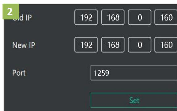
2. Set both old IP and new IP to the camera IP address you want to control, the corresponding communication port to 1259 on mini-pro, configuration path: M(Menu) → FX → PTZ Camera Setting Port on the control software of mini-pro.
