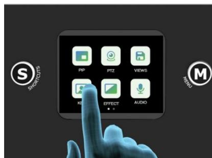
(2) You can choose on or off to enable/disable the function. The sub-screen defaults to input 4, and the main screen defaults to input 1, which can both be changed to other source according to field application.
