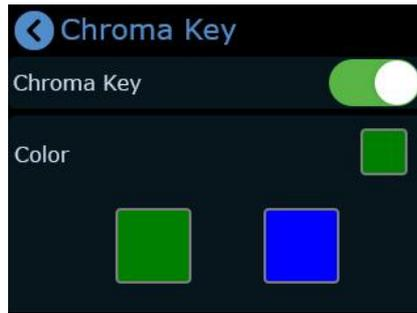
(3) Select the background color which is default in green to be removed and make adjustments. Similar to PIP, the size, position and cropping of the main/sub-screen can be set.
