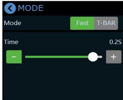
When T-Bar is enabled, all operation could be checked on PST window. Slide T-Bar to switch between PST and PGM.
