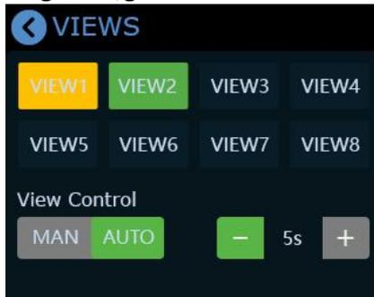
(3) Push button【S】to enter the Shortcut menu where there are buttons of View 1~4 which can loaded directly.
