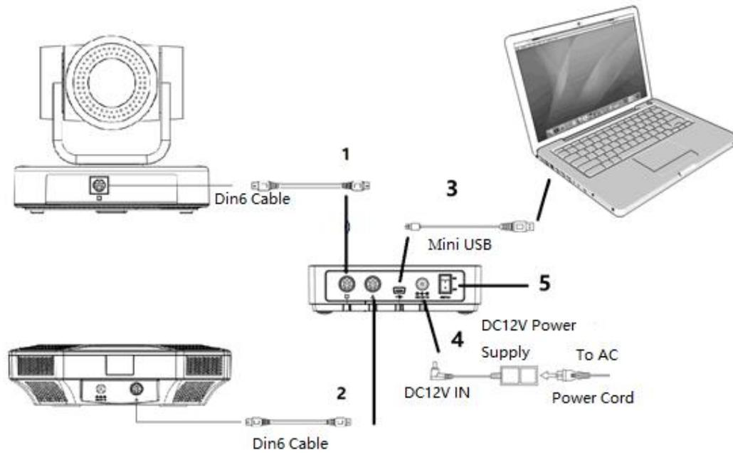
1. Connect camera and hub with original DIN6 data cable
