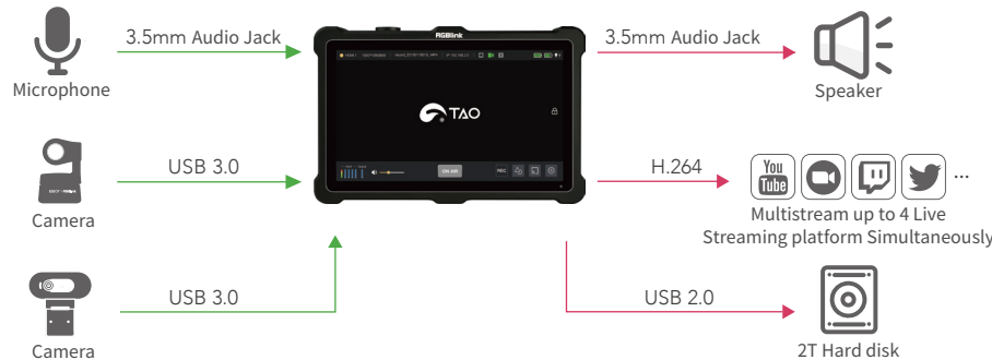
Scene 2: Seamless switching between different USB inputs
