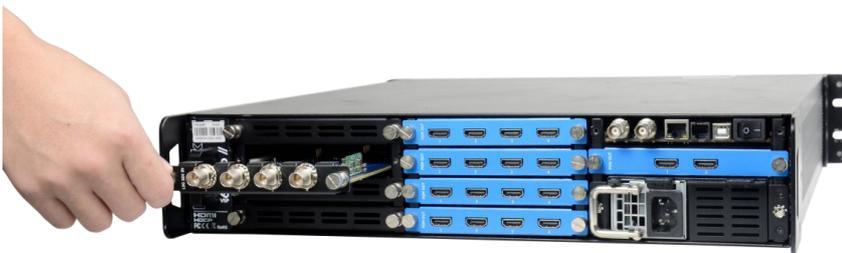
3. Pushing back the input module, as shown in figure:
