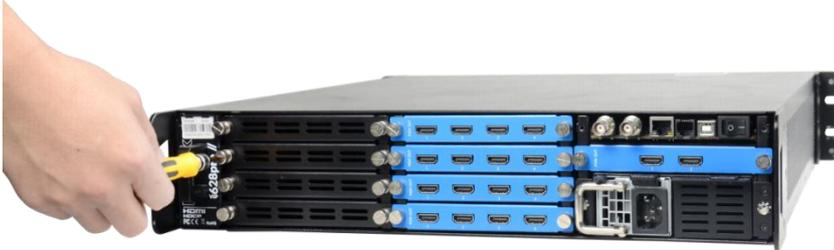
2. Pulling out the input module, as shown in figure:
