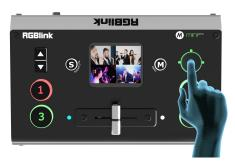
On the PTZ menu interface, when the PTZ function is enabled, the rotation angle of the PTZ can be adjusted by the joystick, and the focal length adjusted by the toggle.
