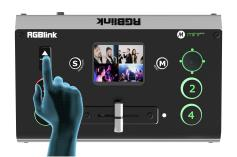
Adjust the size of the screen through the **toggle**, and all the re-adjusted settings will be saved to the current View in real time.
