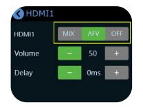
Turn on [MIX] to always add audio to PGM, Turn on [AFV], the audio follows the video switch to perform a soft gradual transition when video is switched.
