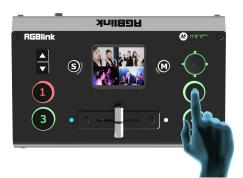
mini-pro is default 0.5S Fast Fade mode, by pushing ①②④signal buttons, 4 input signals can be switched in fast fade mode.
