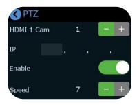
You can choose on or off to enable/disable the function, select the number of camera, and set the IP address.
