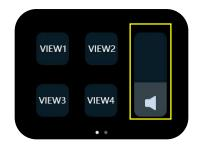
Press button [S] to enter Shortcut interface, adjust the volume by sliding the bar.
