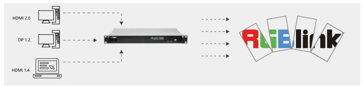
Each of the four outputs may be configured individually with rotation in 1 degree positioning . Video layered and mapped across the output displays.
