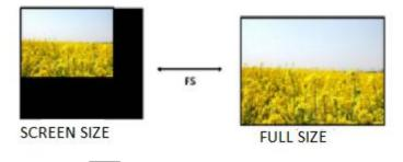
Note: Users can also set <SCREEN> by  $[FS]^{4}$ . Push FS button light on, Led display image in screen size, Push [FS] again, button light off, Led display image in full size.
