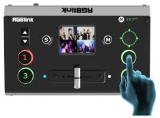
mini-pro is default 0.5S Fast Fade mode, by pushing ①②③④signal buttons, 4 input signals can be switched in fast fade mode.
