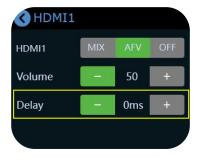
If the sound and the video are not synchronous, increase or reduce the Delay value under AFV.(External and HDMI input audio support delay up to 160ms)
