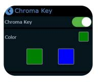
You can choose on or off to enable/disable the function and select the background color to be removed and make adjustments.
