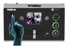
Adjust the size of the screen through the **toggle**, and all the re-adjusted settings will be saved to the current View in real time.
