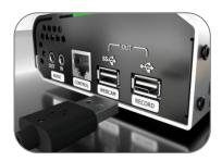
Format the SSD or U-disk and then insert it into the USB2.0 interface RECORD.
