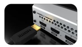
Connect mini-pro HDMI OUT port to monitor to HDMI preview the input and output.
