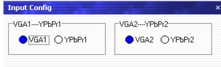
Define VGA1 and VGA2 Input source types, VGA input compatible with YPbPr.
