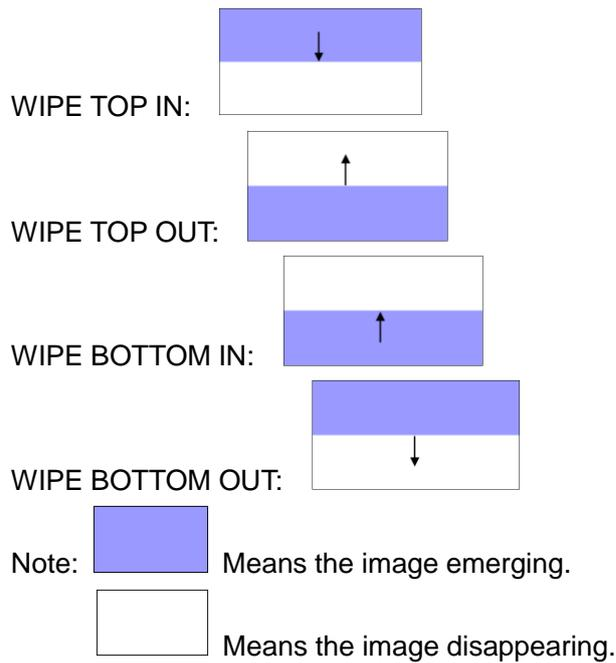
Arrows represents the direction of the image move, that is, the image that arrow point, is compressed or stretched to the direction that arrow indicates, until disappear or full screen.
