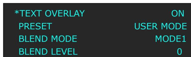
3. Push the **MENU** button, return to [TEXT OVERLAY], turn the knob, OLED screen displays menu options, select 13 modes in PRESET, or select BLEND MODE, which includes two modes:
