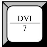
DVI input selection button, its LED light turns on, output will be switched to this channel.
