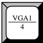
VGA1 input selection button, its LED light turns on, output will be switched to this channel, (compatible with YPbPr).
