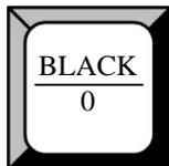
Black button, its LED light turns on, default setting of the test pattern. Test pattern can be set and selected from OLED menu, push the button again, to disable pattern.
