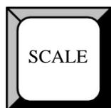
Scale function button: for image size adjustment, push the button to enter the scale menu. Turn the knob to select the relevant submenu. For details, please refer to [MENU](#) in menu orientation and [How to Set the Size and Position of the Single Image](#).
