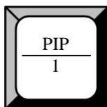
PIP function button: Single image or dual image selection button. Push the button, its LED light turns on, and PIP function is open. Push the button again, its LED light turns off, and close the PIP function, change to single image. OLED shows as follows:
