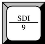
SDI input selection button, its LED light turns on, output will be switched to this channel.
