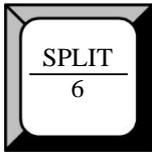
Split function button: push the button, its LED light turns on, split function is open. OLED menu shows as follows:
