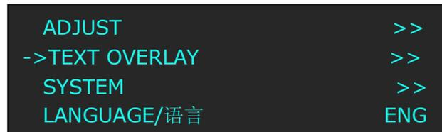
2. Turn the knob, choose “TEXT OVERLAY” option, choose ON, and enable the TEXT OVERLAY function.
