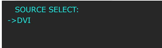
CV1 button light turns off after pushing DVI button. DVI button light will be on if the DVI signal is effective and stable. And if the DVI signal is invalid or no input, DVI button light will flash.
