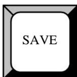
Save button: push it to enter **SAVE** mode, turn the knob or push the number button which light up to save.
