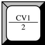
CV1 input selection button, its LED light turns on, output will be switched to this channel.
