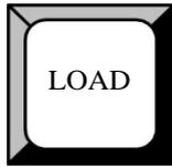
LOAD button: push it to enter **LOAD** mode, turn the knob or push the number button which light up to load the saved parameters.
