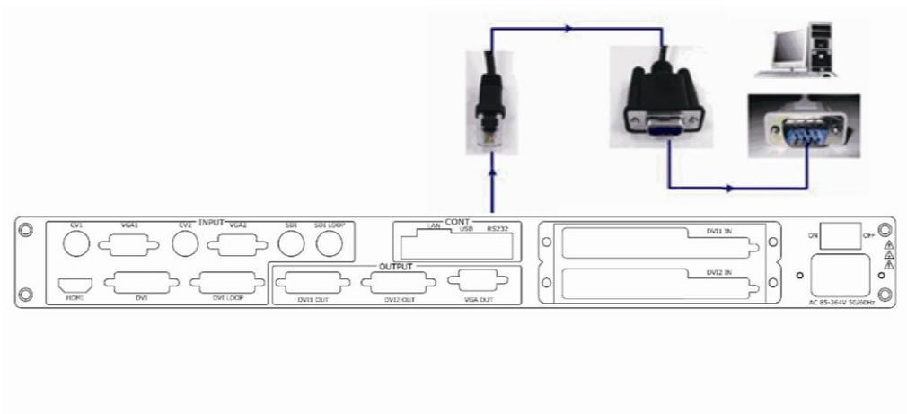
There is no any serial port on your PC, you will need another Serial to USB adapter. Connect one end of the RJ11 download line to the RS232 on the video processor. Connect the end of USB-side to the PC; Ensure the cable connection is good. Turn on the Video Processor VSP 198CVS.
