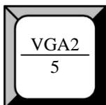
VGA2 input selection button, its LED light turns on, output will be switched to this channel, (compatible with YPbPr).
