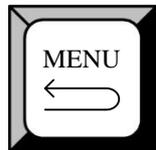
Advanced menu button: push the button to enter the menu items. Turn the knob to select the relevant submenu. For details, please refer to [MENU](#) in menu orientation.
