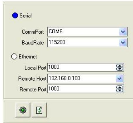
Check and tap [Serial], Serial Port , for example, is **COM6** which is checked from device manager. Set VSP 198CVS Boud Rate to be :115200, Click [Confirm] after setting.
