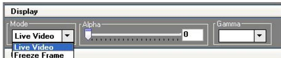
Display toolbar Users can set Alpha value of “dynamic Video” and “static current frame” through display toolbar. When it is in dynamic Video, the video plays properly; when it is in static current frame, the video stop playing.
