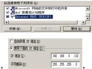
, Now we can revise the equipment IP address to the same band with that of computer **192.168.0.XXX;**
