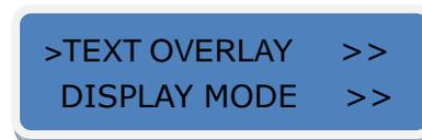
3. Turn the knob, choose TEXT OVERLAY mode, choose ON, TEXT OVERLAY function open.
