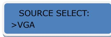
CV1 button light turns off after pushing VGA button. VGA button light is on if the VGA signal is effective and stable. And if the VGA signal is invalid or no input, DVI button light will flash.
