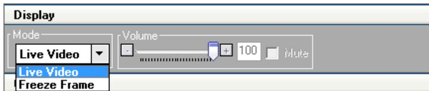
Display toolbar Users can set Alpha value of “Live Video” and “Freeze Frame” through display toolbar. When it is in Live Video, the video plays properly, when it is in Freeze Frame, the video stop playing.
