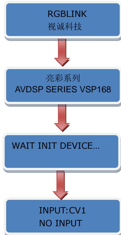
4. After start, the equipment is default load SAVE1 parameter, CV1 key light is on, and the device is in normal working.
