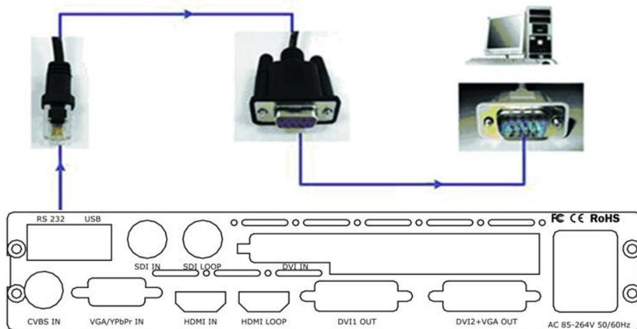
Ensure the cable connection is good. Turn on the VSP 168S Video Processor.
