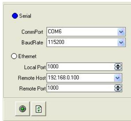
Check and tap [Serial], Serial Port, for example, is **COM6** which is checked from device manager. Set VSP 168S Boud Rate to be :115200, Click[Confirm] after setting.
