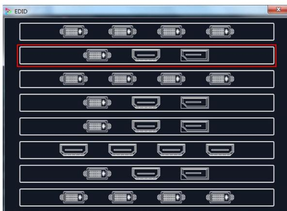
Click the input port, and set the width, height and frequency. Click "Set" after setting. Select "Reset", all the setting will be recover to factory setting.
