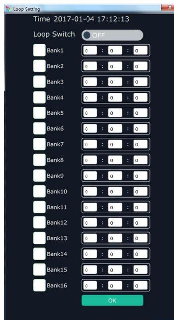
Slide the loop switch to enable or disable the loop function for the bank. If select "ON", the bank play time can be set.
