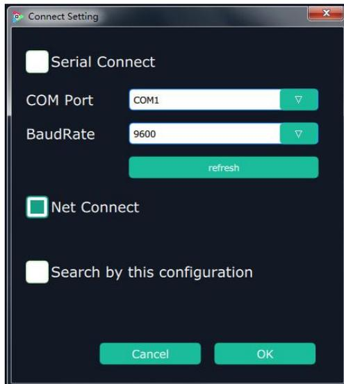
Select the serial connect and net connect, the software will search all the devices if not select “Search by this configuration”.
