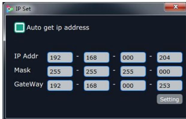
Default “Auto get ip address”. Users can also set IP address, mask and gateway manually. This is usually used if one computer control some devices or remote control. It takes effect after reboot the software if change IP through network.
