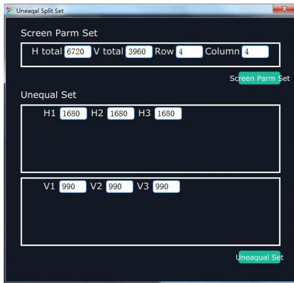
Set H1, H2, H3, V1, V2 and V3. For example, set H1 as 960, H2 as 1920, H3 as 960, V1 as 800, V2 as 1080, and V3 as 1000, the layout is shown in the figure below:
