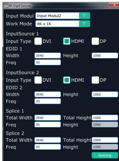
2. Open the videowall mode, it will display the combined HDMI signals in the signal list, shown as follows:
