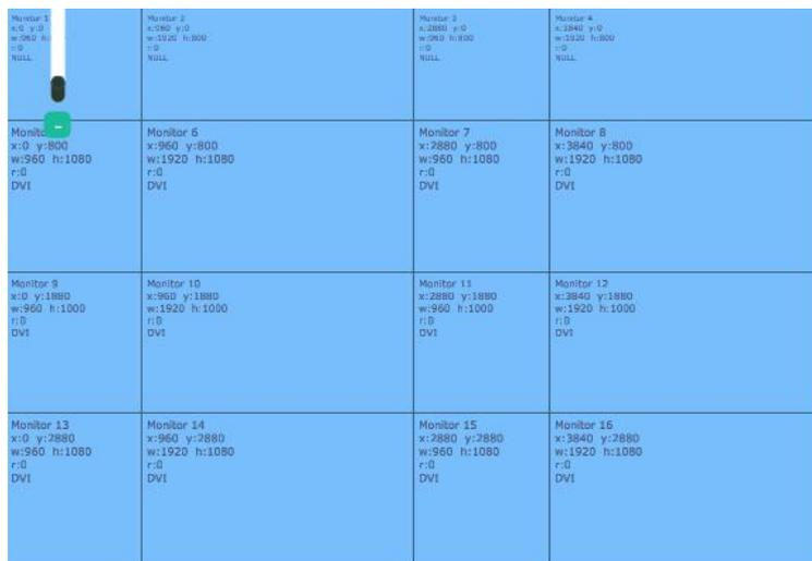
LCD Type: Slide the monitor type switch, and select "LCD Type". Besides H total, V total, row and column, user can custom the top border, bottom border, left border and right border in LCD type, as shown in the figure below:
