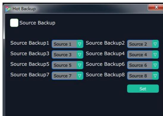
Enable the hot backup function, as shown in figure
