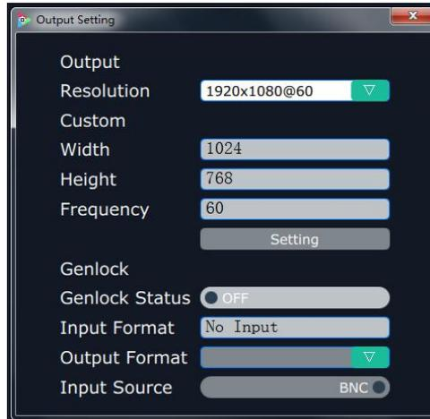
**Output:** Click the drop down arrow after the format, and select the output resolution in the pull-down menus according to actual need.
