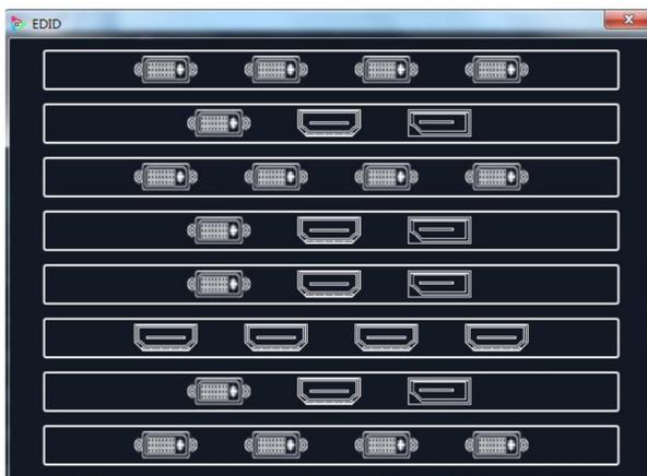
The special display project or LED display application would like to require special resolution settings to meet the requirement. Select the input or output board to read and write the EDID. As shown in the figure below:
