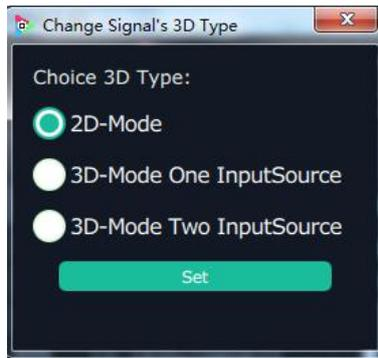
User can select “3D-Mode One InputSource” or “3D-Mode Two InputSource”. If select “3D-Mode One InputSource”, it will show “3D” on the signal, as shown in the figure below:
