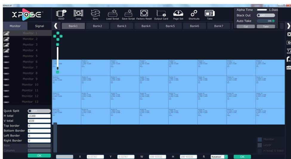
In videowall mode, there are max 32 image in the output interface, group of two outputs, one output module can display 8 images.
