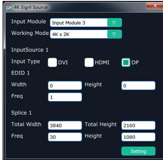
**Input Module:** Click the pull down arrow to select the 4K input module.
