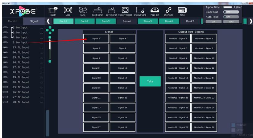
**Note:** Click the monitor (the border of the monitor will turn to red), then double click the signal (the border of the monitor will turn to yellow), the signal will be switched to the monitor.
