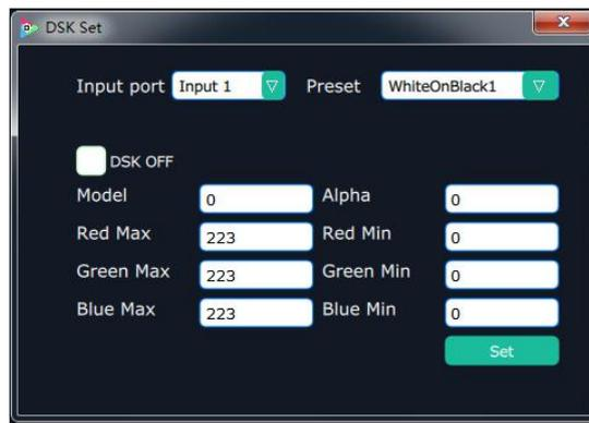
Select DSK ON, as shown in figure
