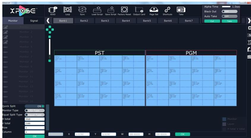
In preview mode, all the settings are displayed in the PST monitor, click “Take” or “Cut” in “Take” box to seamless switch the signal to LED display. If select “Auto Take ON” or “Black Scene ON”, the preview image will seamless switch or black to LED display instantaneously.
