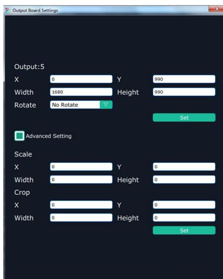
If user need to connect to the LED display, or there is deviation in splitting, enter to the advanced setting, and scale or crop the image.
