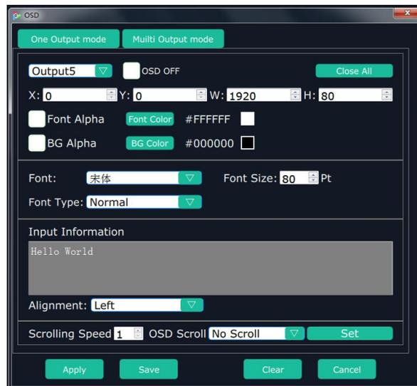
**Output Mode:** One output mode or more output mode can be selected. In one output mode, user need to enable the OSD function and select the output first. The operations are as follows:
