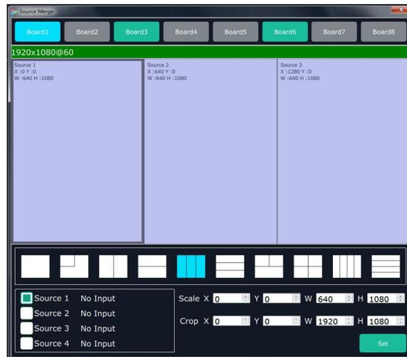
Click any layer, then click any source, and the layer source can be switched, as shown in the figure below:
