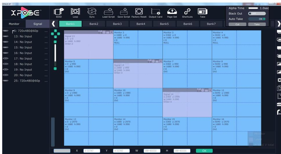
**Adjust Layer:** Two ways can change the size and location of the opened layer:
