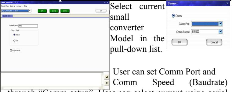
Select current small converter Model in the pull-down list.
