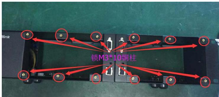
Step 2: Lock M3\*5 cross countersunk head screw in the position as the the red arrow pointed in the following pic.
