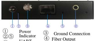
Connect one end of the power adapter with the device, the other end into a socket. Plug in, red power indictor light means the device works normally.
