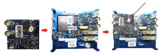
Step 4: When SDI input module installation complete, assemble the two circuit boards, and lock the rear panel, adding SDI input module finished.
