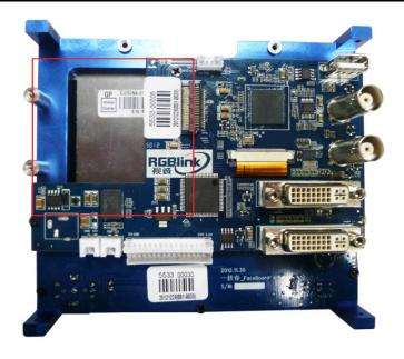
Step 3: Install the SDI input module in the area as shown above, then tighten the screws, install it one by one.
