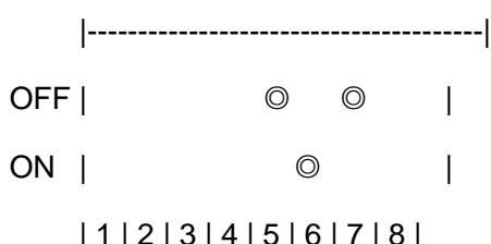
10. Dial switch 5, 6 OFF, dial switch 7 ON: SDI output resolution is 576i 50Hz.
