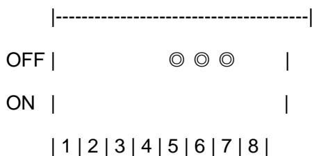
12. Dial switch 8 OFF: AES/EBU output, no analog audio output.
