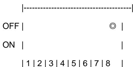
13. Dial switch 8 ON: L-analog and R-analog audio output, no AES/EBU output.
