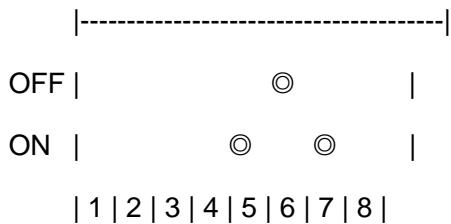
7. Dial switch 5 ON , dial switch 6, 7 OFF: SDI output resolution is 1080i 50Hz.
