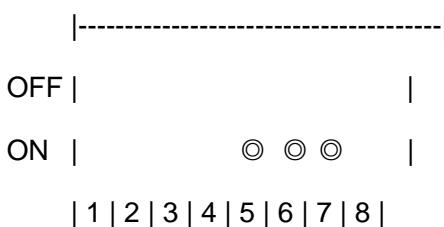
5. Dial switch 5, 6 ON, dial switch 7 OFF: SDI output resolution is 1080p 50Hz.
