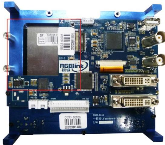
Step 3: Install the SDI input module in the area as shown above, then tighten the screws, install it one by one.
