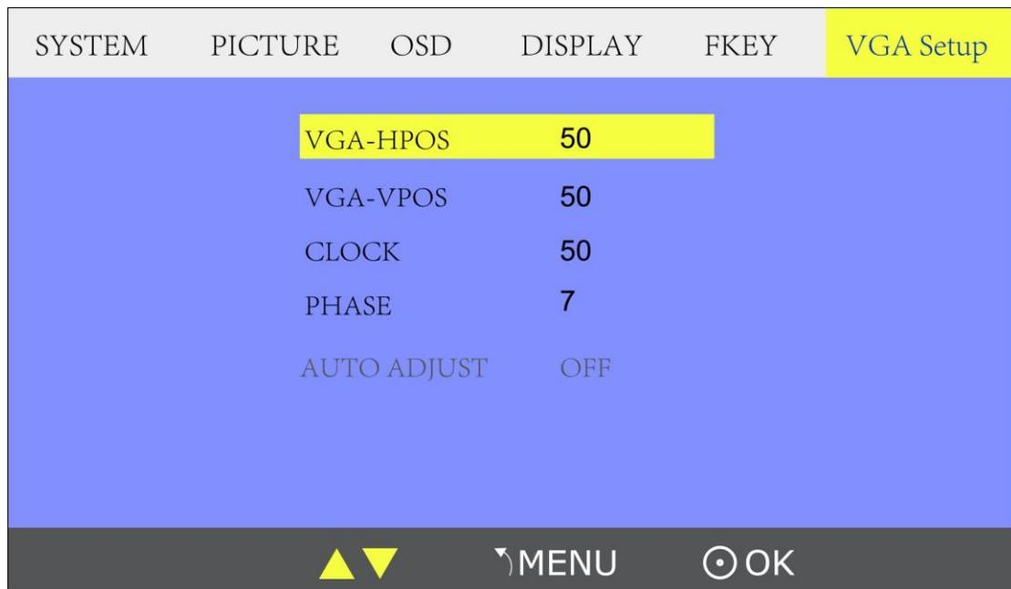
Enter to “VGA Setup” submenu to adjust VGA-HPOS (0~100), VGA-VPOS (0~100), CLOCK (0~100), PHASE (0~100). Also can select “ON” at “AUTO ADJUST” to adjust when input VGA signal.
