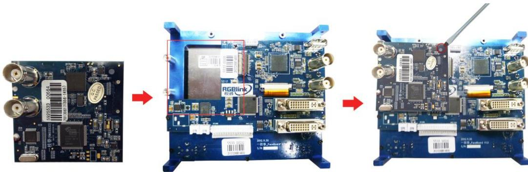
Step 4: When SDI input module installation complete, assemble the three circuit boards.
