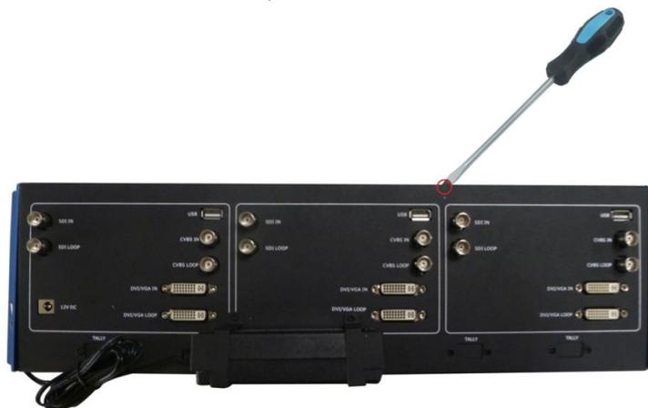
Step 2: Take three circuit boards inside apart respectively, the red box in circuit board is the area for SDI input module installation.
