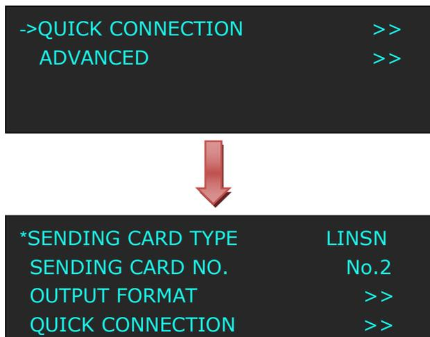
(6) Turn the knob, select <SENDING CARD NO.>, push the knob to confirm. Turn the knob and select “No.1”, push the knob to confirm. Shown as follows:
