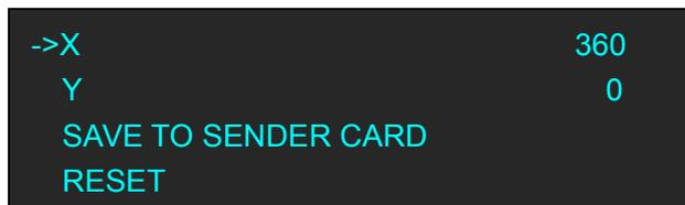
(12) Same as above, set X of Port D of No.2 sending card as 360. Then connect the Port D and Port U of Two Sending Cards to LED Screen is finished. Rendering is as follows:
