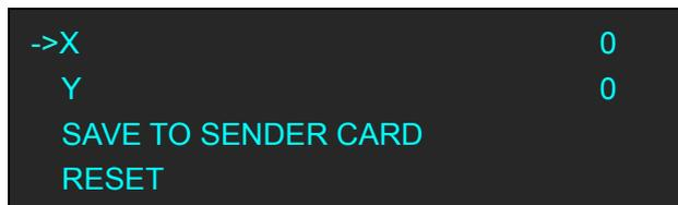
(11) Turn the rotary knob, and select <X>, set X as 360 (Note: X=HORIZONTAL CARD×WIDTH, in the previous part, we set horizontal card as 3 and width as 120). Shown as follows:
