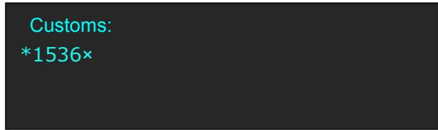
6. After the digital, push the knob will add \*, means before the \* is the horizontal size. Same operation for vertical size, for example input 1536 as following:
