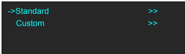
3. Default <Standard> option, push the knob to confirm. Turn the rotary knob, and select the output format according to actual needs.
