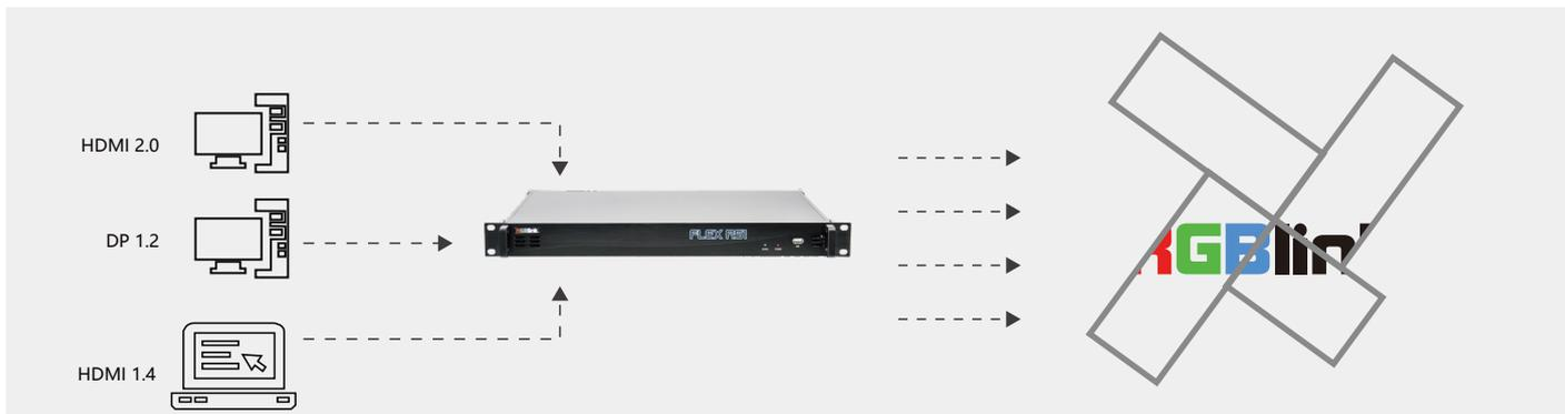
Each output can be configured independently allowing displays of multiple sizes and pixel densities to be supported
