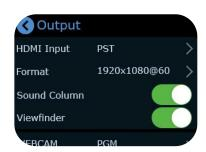
HDMI output defaults multi-screen preview, which can be switched to PGM or the 4 input content in field application.
