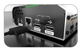
Connect the laptop to mini-pro's USB 3.0 port via USB cable, and mini-pro will be captured as a webcam source.
