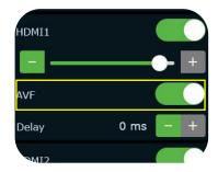
Turn on AFV, the audio follows the video switch to perform a soft gradual transition when video is switched.
