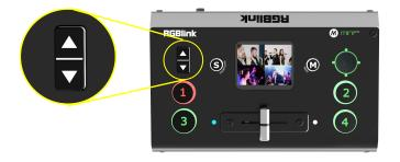
When the touch screen is in the main interface/ preview interface/Shortcut interface, the PGM audio volume can be adjusted by the **Up/Down keys**.
