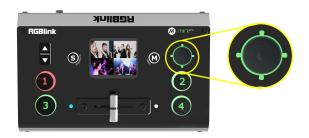
You can use the joystick to switch the selection of the main/sub-screen and adjust the size, push the signal source to switch between different signals.
