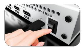
Push the Power button on the rear panel, the device will enter to the boot interface within 10S.
