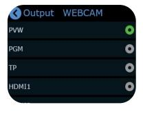
USB 3.0 output recognized as WEBCAM on computer defaults to be PGM which can be changed to multi-screen PST or TP (Test Pattern).
