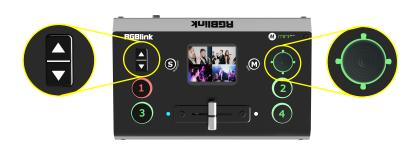
On the PTZ menu interface , when the PTZ function is enabled, the rotation angle of the PTZ can be adjusted by the joystick, and the focal length adjusted by the Up/Down keys.
