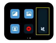
Press button [S] to enter Shortcut interface, adjust the volume via sliding the bar
