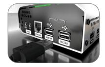
Format the SSD or U-disk and then insert it into the USB2.0 interface RECORD.
