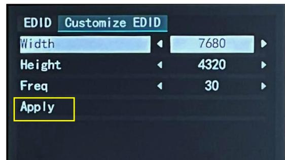
**Note:** The resolution on the signal source (such as a computer) needs to be same as the D8. Refer to <User Manual> for details.
