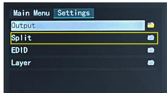
Select layout, then set parameters, such as H Total, V Total of screen according to actual need. Use the numeric keyboard to enter parameters, then click "Save Settings" > "Confirm" to save above settings.
