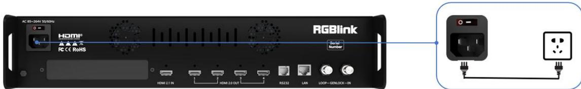
Connect power and D8 with standard Power Cord. Plug one end of the power cable to the D8's power interface. The other end is connected to the power socket.
