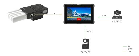
Step 1: Plug a Dongle with SIM card inside to USB port.
