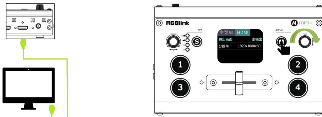
Connect LCD display to mini+ by HDMI cable to display 6-picture PVW.
