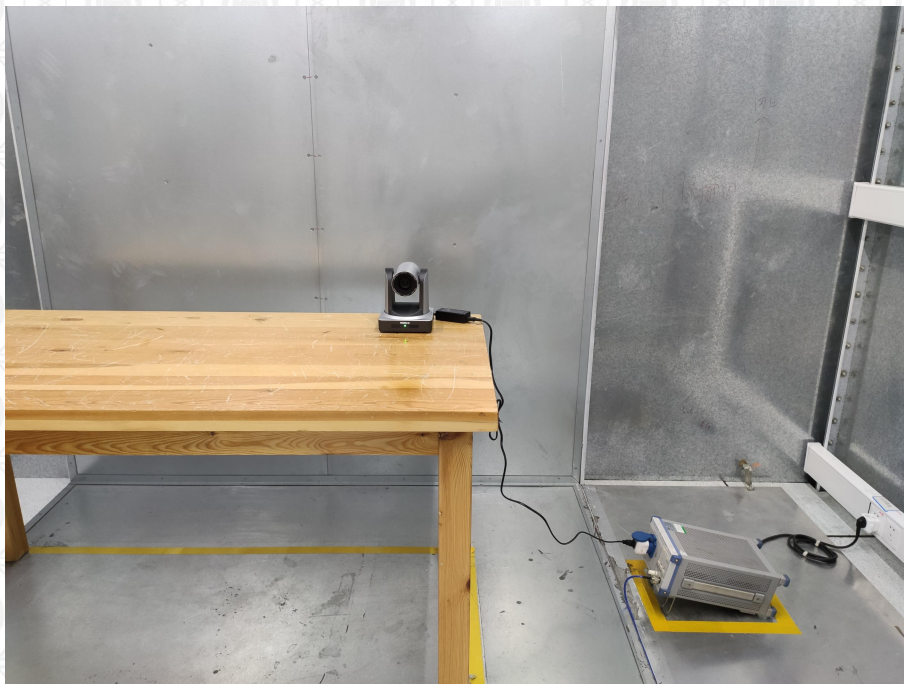
Figure 6: Conducted Emission Test Setup
