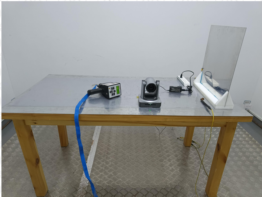
Figure 9: Electrostatic Discharge Test Setup
